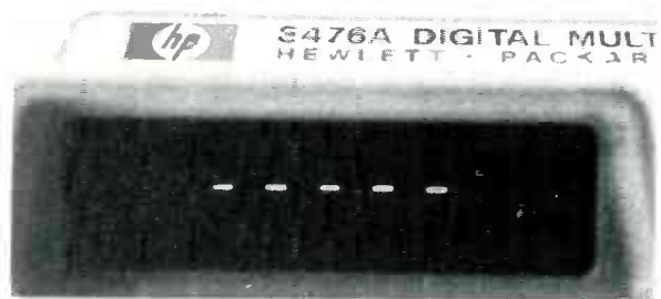
Fig. 4 A series of non-flashing dashes indicates overload or overrange.
