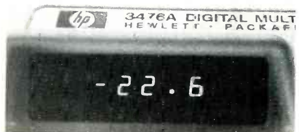
Fig. 5 Negative voltages produce a minus sign before the readout; no indication is used for positive voltages or currents.
