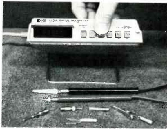
Fig. 7 Some of the screw-in tips for the test prods are shown here.
