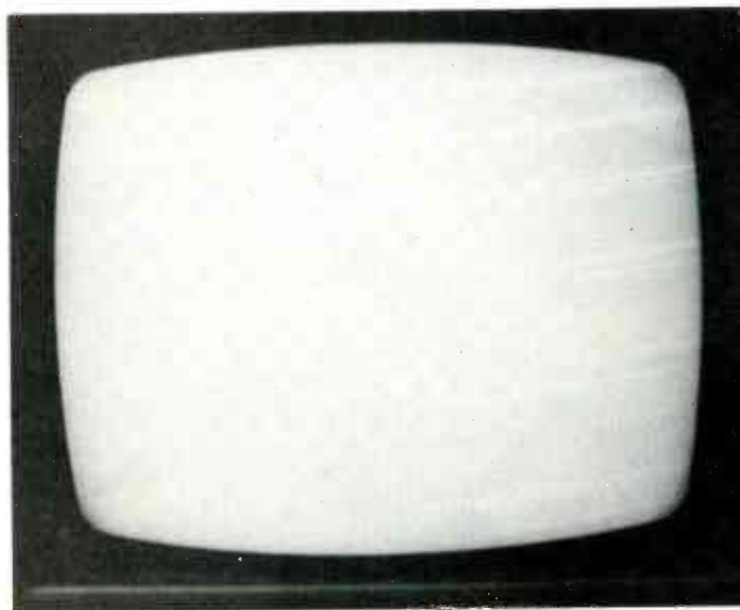
Fig. 1 The main visual symptom was a bright raster without any picture. Other video troubles can black out the screen. Whatever the brightness condition, it can provide valuable clues about where to look.
