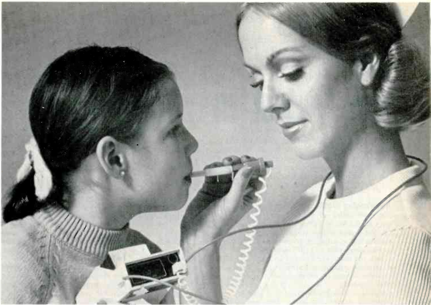
An IVAC electronic thermometer measures a patient's temperature in about 15 seconds, with the exact temperature shown by a digital readout. The probe covers are made of plastic, and a new one is used for each patient. (Courtesy of GTE-Sylvania, Inc.)
